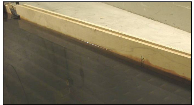
Figure 4: Bending of foil through steel net
