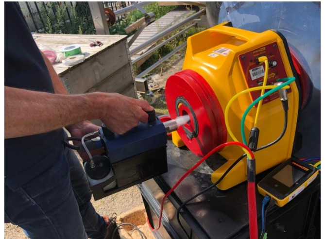
Blowing smoke through the fan
