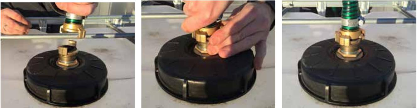
water hose connected to IBC container via quick coupling
