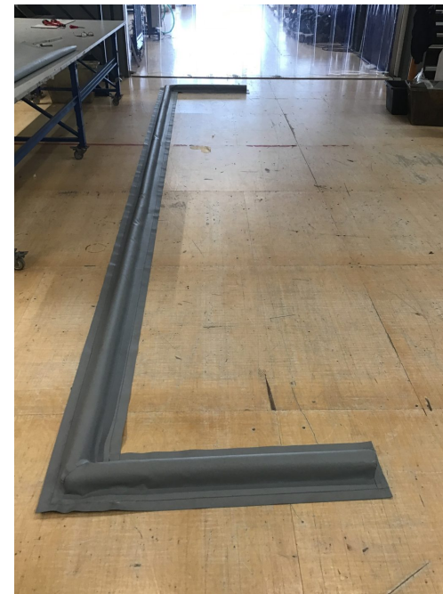
U-shape with two welded-in 90° corners, ready to be laid into the sealant
