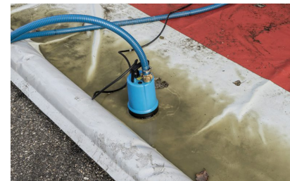
The flat suction pump discharges the wash water to your separator or buffer.
