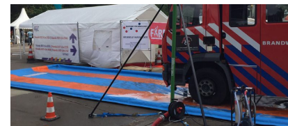
Portable wash pad in use.
